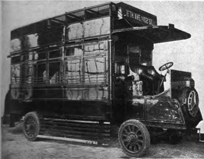
Fifth Avenue bus equipped with safety fender to guard against pedestrians walking into rear wheels
